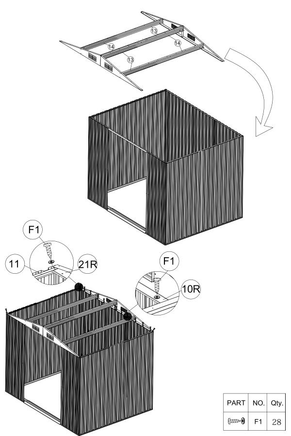
Place the roof panels (P5),(P6) on the top of Gable panels and roof supports Line up the boles and secure with (F1) bolt and nut with washers.
