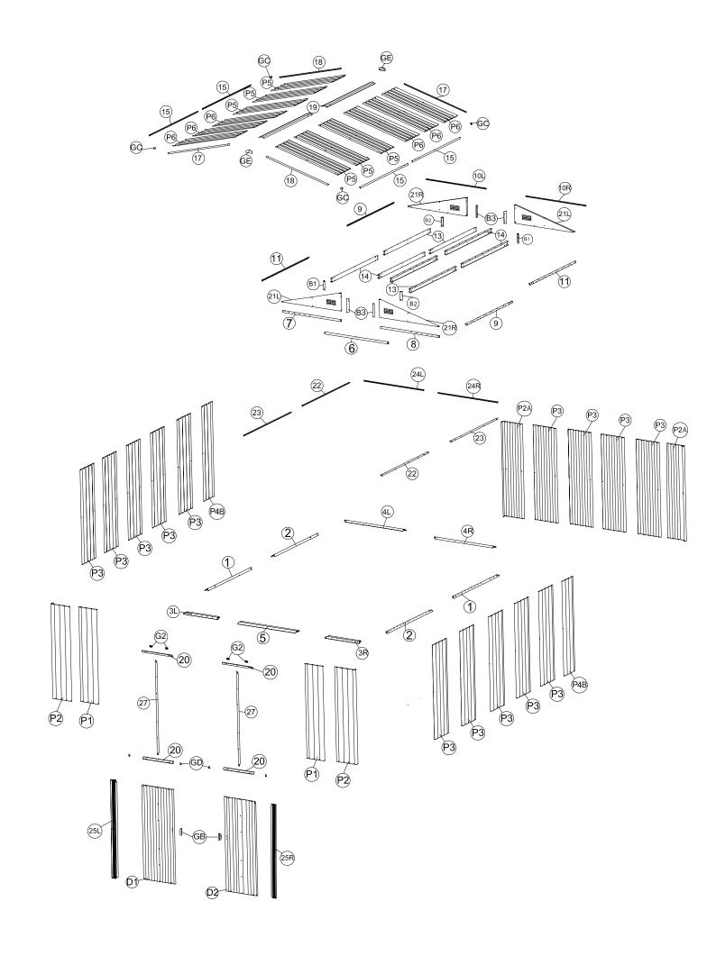
Assemble base bars from (1) to (4R) with (F1) Screws. Then place the entrance taper channel (5)on top of the bar(3L) and(3R). Secure with (F1) screws to the foundation. Seeing the following figures .Make sure the base bar assembly in a perfect square.
