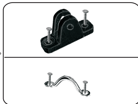
10. Drill and secure the deck mounts and saddles with self tapping screws.
