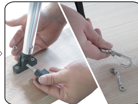
11. Assembly main bow tube and rear support pole onto deck mount with thumb screws and nuts. Attached the hook of the front adjustable strap onto saddle.
