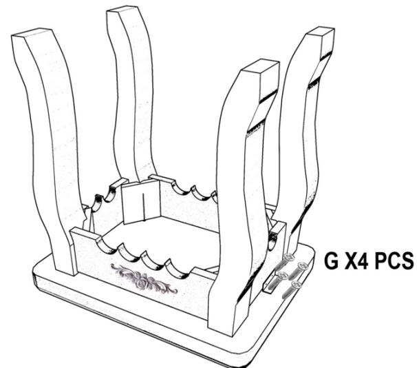
USE THE HARDWARE **F** AND SCREW **G** TO CONNECT THE MAT TO THE FRAME.
