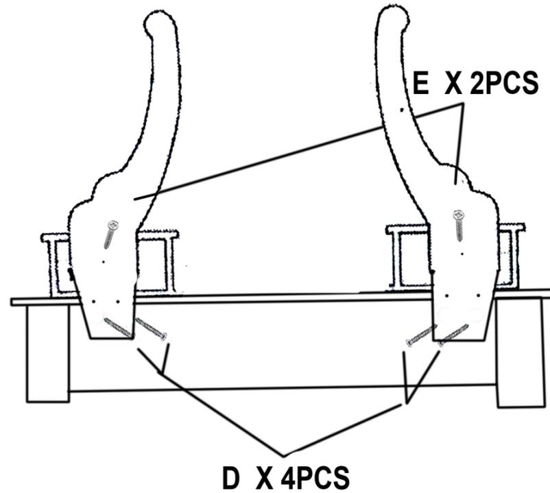
USE THE HARDWARE **D** TO MOUNT THE WOODEN PROP TO THE TABLE.
