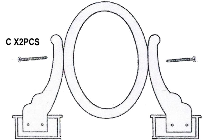
USE THE HARDWARE **C** TO CONNECT THE MIRROR TO THE WOODEN PROP
