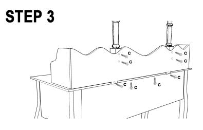
INSTALL THE COMPONENTS INSTALLED IN STEP 2 ONTO TABLE BODY(12). THEN INSTALL MIRROR FIXTURE(3) ONTO THE ASSEMBLED COMPONENT OF STEP 2. USE SCREWS C(X8PCS)
