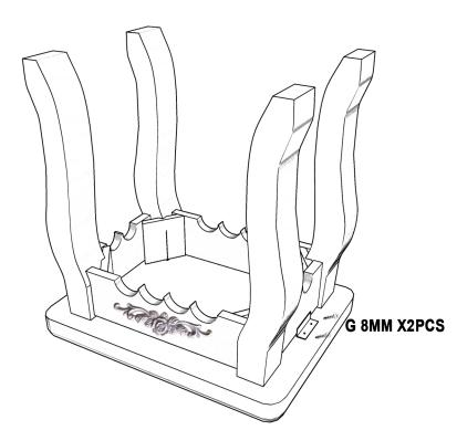
USE THE HARDWARE AND THE SCREW G (X4PCS)TO MOUNT THE STOOL FRAME TO THE CUSHION.
