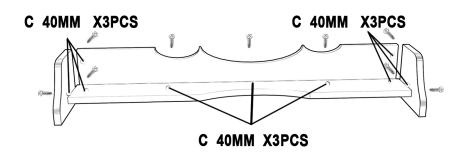
USE SCREWS C(X9PCS) TO CONNECT BOARD (4) BOARD (5) AND BOARD (11) TOGETHER
