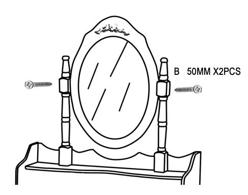
USE SCREW B (X2PCS) TO CONNECT MIRROR FIXTURE (3) TO MIRROR (1)
