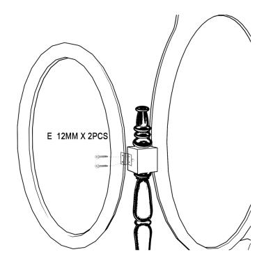
USE SCREWS E(X2PCS) TO INSTALL SMALL MIRROR(2) ON THE MIRROR FIXTURE(3) REPEAT THE STEPS AND INSTALL SMALL MIRROR ON THE OTHER SIDE. THE INSTALLATION IS COMPLETED.
