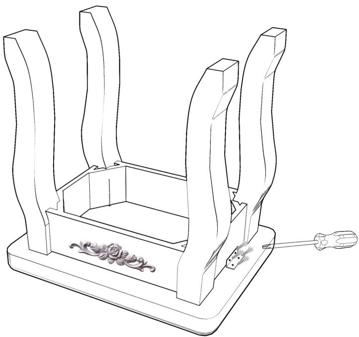
USE THE HARDWARE D (X2PCS) AND THE SCREW E (X8PCS) TO MOUNT THE MAT TO THE STOOL FRAME.
