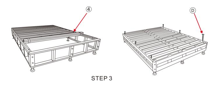
Lock each slat into place by applying pressure.
