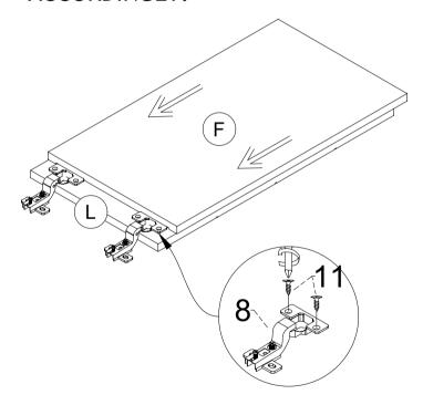
Insert 2x hinges (8) into panel [N]x2 with 4x screw (11).
