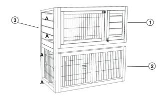
Attach front panel part①, part②to left side panel part③, secure with 4x screw (A).
