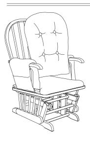
Put back cushion on the backrest. The two belts on the top of the backside of the back cushion should tied onto the bentwood, the other belts could tied on pole of the backrest.
