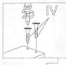
Attach panel [P] into base panel of drawer screw with 4x screw (IV).
