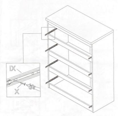
Attach 4x slide rails (IX) in place on each of the panels [A] [H] using 3x 12mm small screws (X) in each rail bracket. Fasten all screws.
