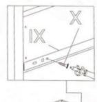
Attach 2x rail component (IX) to both left and right of the drawer using 3x screw (X) in each rail.
