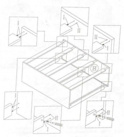
Insert 6x pin (II pin) into panel [H] and 10x dowels (I) into corresponding holes in panels [B] [C] [D] [E]x3 [F] [G]. Slot together with side panel [H]. Place 6x locking nuts (II nut) into holes in connecting parts and tighten with screwdriver.
