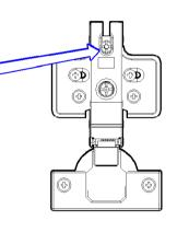
Loosen this screw, adjust by moving back and forth
