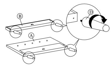
Step 2: Attach side rail (C) to footboard (B) and headboard (A) by pushing the bracket down to fit it.
