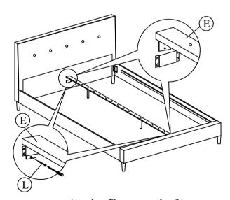
Attention: Please ensure that (L) screw is being attach as per the A.I shown to avoid base being collapse.
