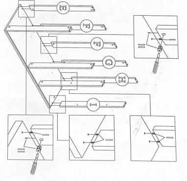
with screwdriver. Place 4x locking nuts (II nut) into holes in connecting parts and tighten holes in panels [E] [F]x2 [G] [H] [I]. Slot together with side panel [A]. Insert 4x pin (II pin) into panel [A] and 8x dowels (I) into corresponding
