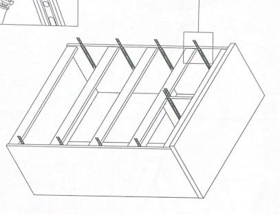
Attach 4x slide rails (IX) in place on each of the panels [A] [K] and 2x slide rails (IX) to both sides of panel [J] using 3x 12mm small screws (X) in each rail bracket. Fasten all screws.
